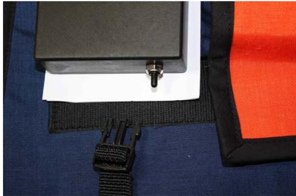
5. The system is switched on / off by plugging in / unplugging the power-supply cable. Switch on the **Warm-Up** system by plugging the power-supply cable into the socket on the top left of the control module. To switch the system off after use, simply unplug the cable.
